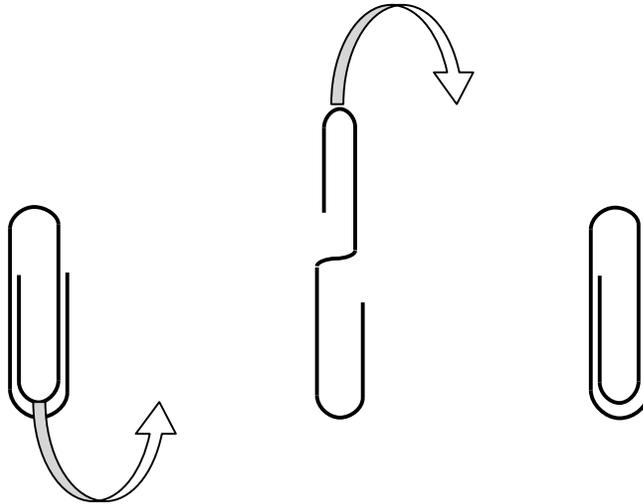
3. Repeat steps 1 and 2 until the paperclip breaks. Record the number of loading cycles that elapse. (Note: if the paper clip breaks mid-cycle, that cycle does not count in the ‘number of cycles to failure’)
